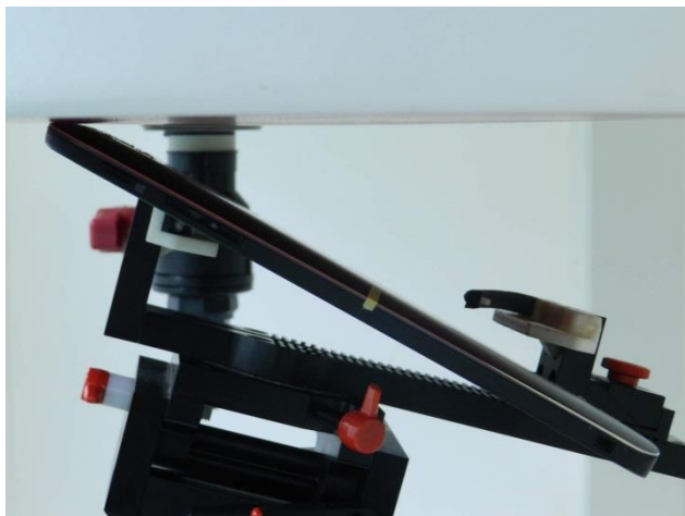
Curved surface of Edge1, Test Separation 0 cm
