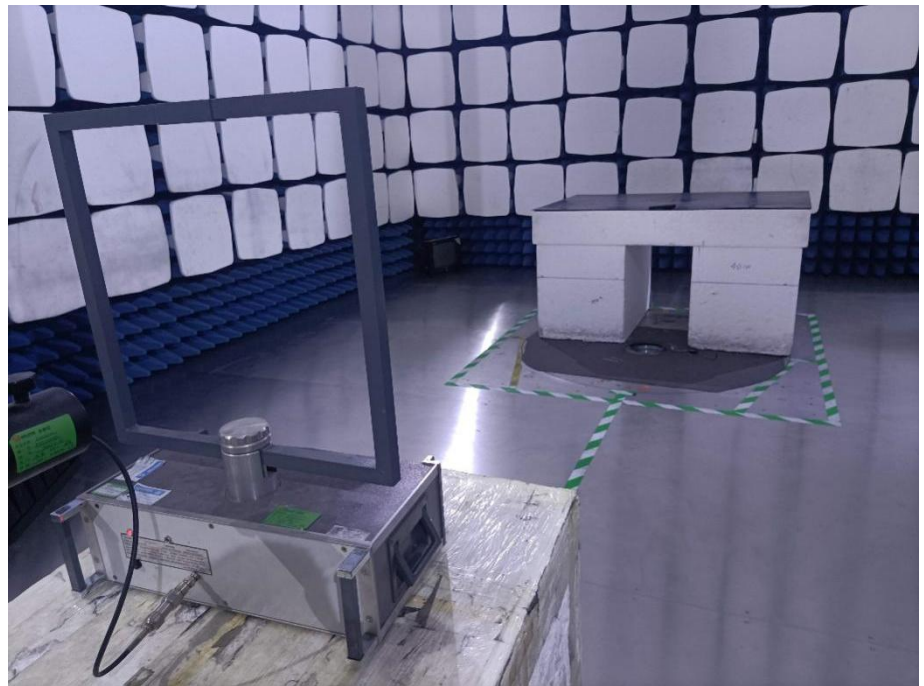
Radiation Emission Test Setup (Below 30MHz)
