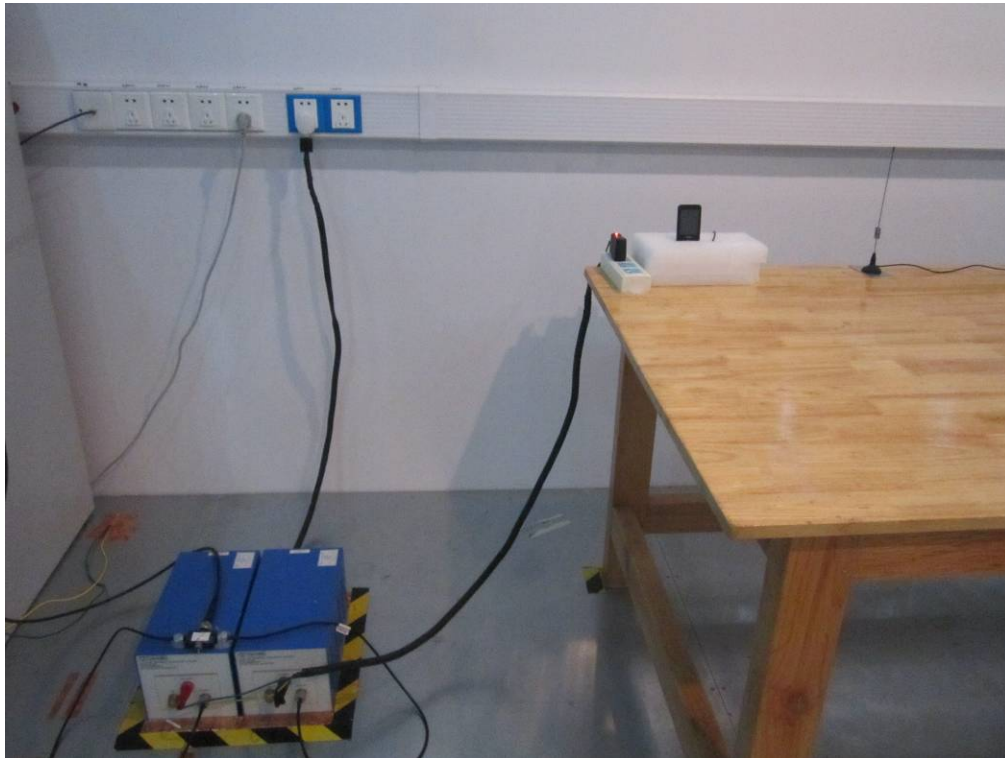
Conducted Emissions Test Setup Front View
