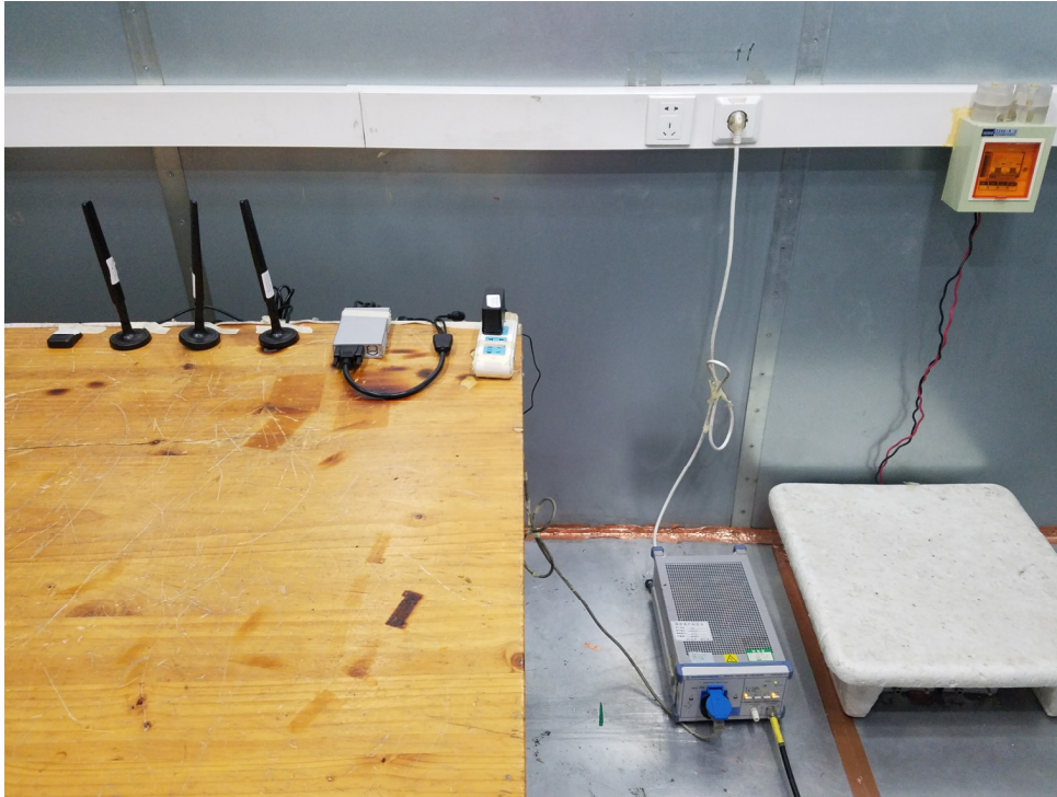
Picture 2: Conducted Emissions Test Setup
