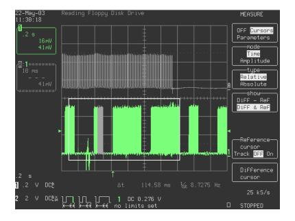
The above plot shows the Morse P transmission in the enclosed box. The dot timing at 55°C is 114.58ms.
