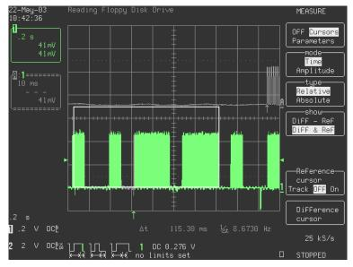
The above plot shows the Morse P transmission in the enclosed box. The dot space timing at -40°C is 115.30ms.
