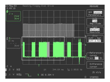
The above plot shows the Morse P transmission in the enclosed box. The dash timing at 25°C is 344.64ms.
