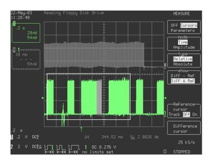
The above plot shows the Morse P transmission in the enclosed box. The dash timing at 55°C is 344.52ms.
