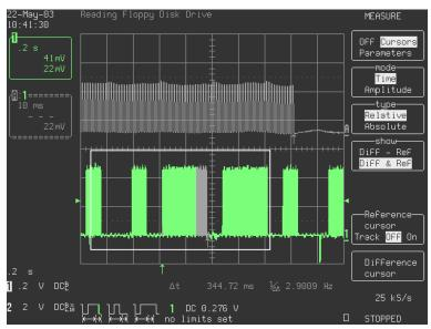
The plot above shows the Morse P transmission in the enclosed box. The dash timing at -40°C is 344.72ms.
