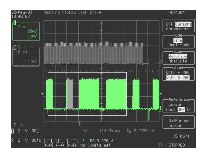
The above plot shows the Morse P transmission in the enclosed box. The dot timing at -40°C is 114.60ms.
