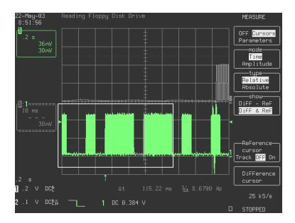
The above plot shows the Morse P transmission in the enclosed box. The dot *space* timing at 25°C is 115.22ms.
