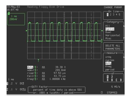
The plot above shows the Modulation duty-cycle for the Fastfind Plus with Morse P transmission. The modulation frequency is 1kHz.
