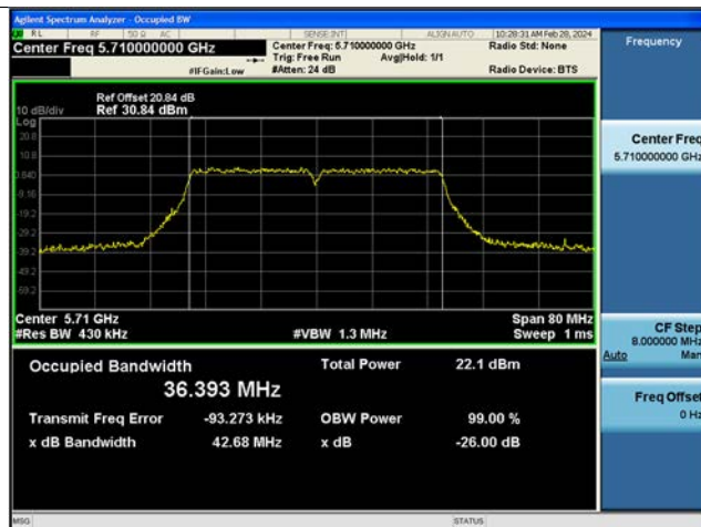
802.11ac(VHT40) 26 dB Bandwidth (CH 142)
