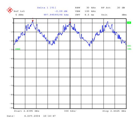
The hopping channel carrier frequencies are separated by a minimum of the 20 dB bandwidth of the hopping channel.
