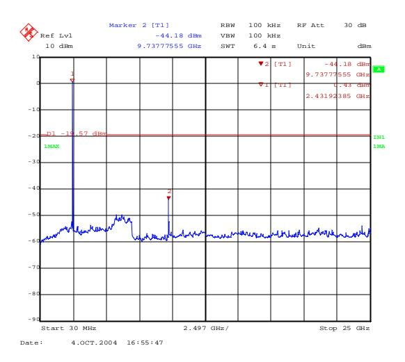
Note: The peak above the limit is the carrier frequency. Verdict: PASS
