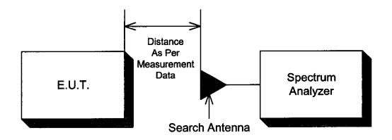
FCC PART 15, SUBPART C INTENTIONAL RADIATORS USED AS FIELD DISTURBANCE SENSORS PROJECT NO.: 9R01681.1
