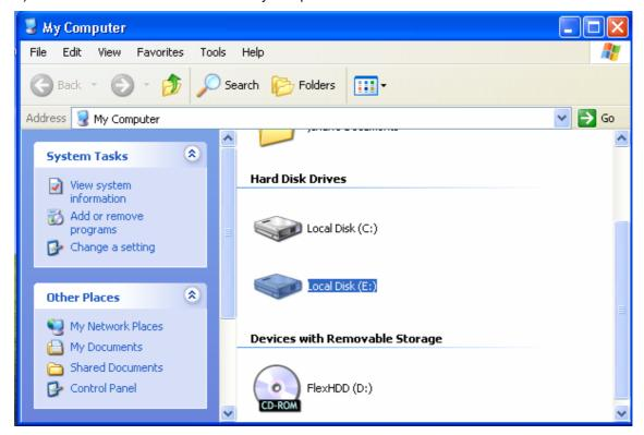
\*\* Caution: The new hard disk which doesn't have FDISK and FORMAT, can not be recognized in "my computer"
