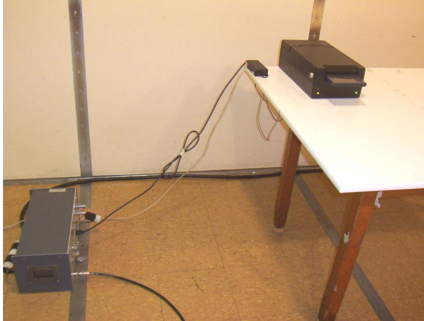
Conducted Emission Test Setup
