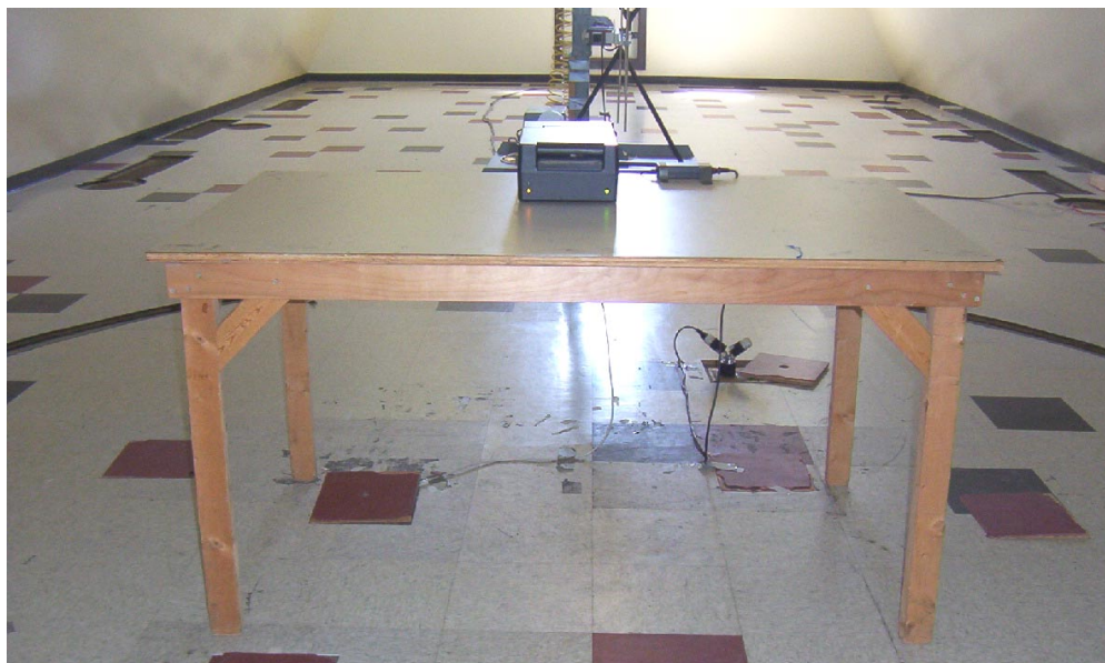
Radiated Emission Test Setup (Front)
