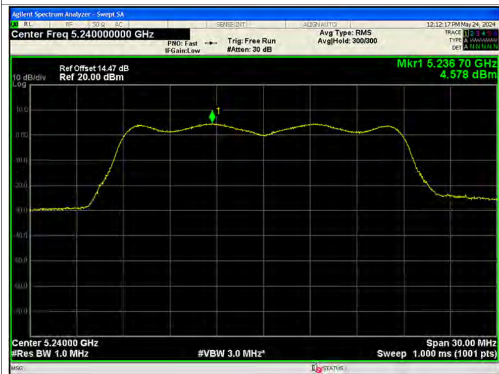
PSD NVNT n20 5260MHz Ant1
