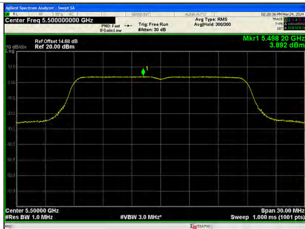
PSD NVNT n20 5500MHz Ant2
