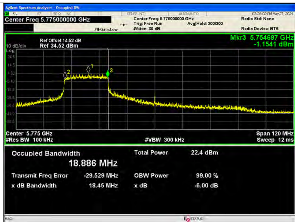
-6dB Bandwidth NVNT ax80 242@61 5775MHz Ant2
