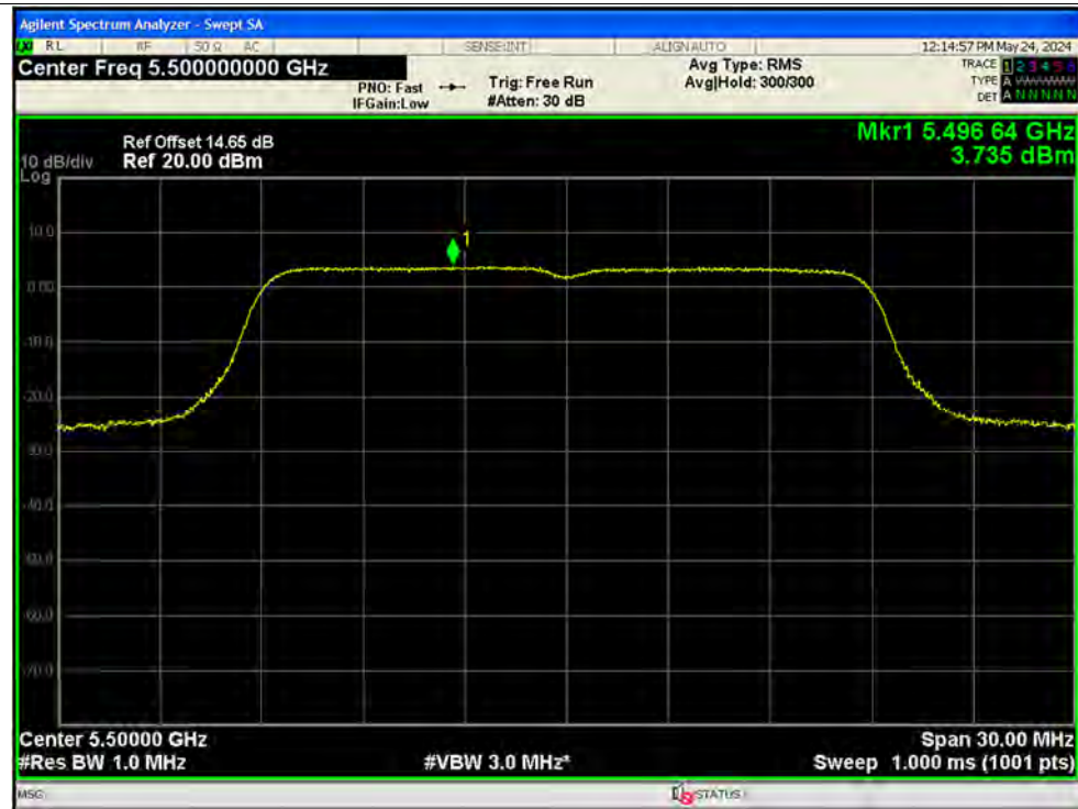
PSD NVNT n20 5580MHz Ant1
