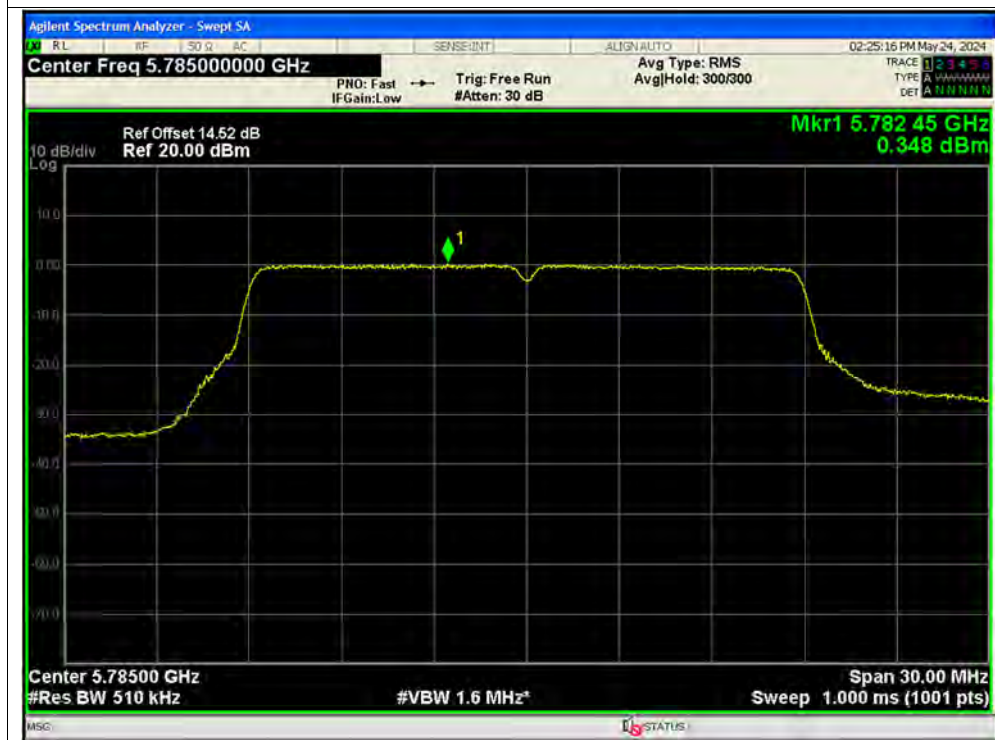
PSD NVNT n20 5825MHz Ant2
