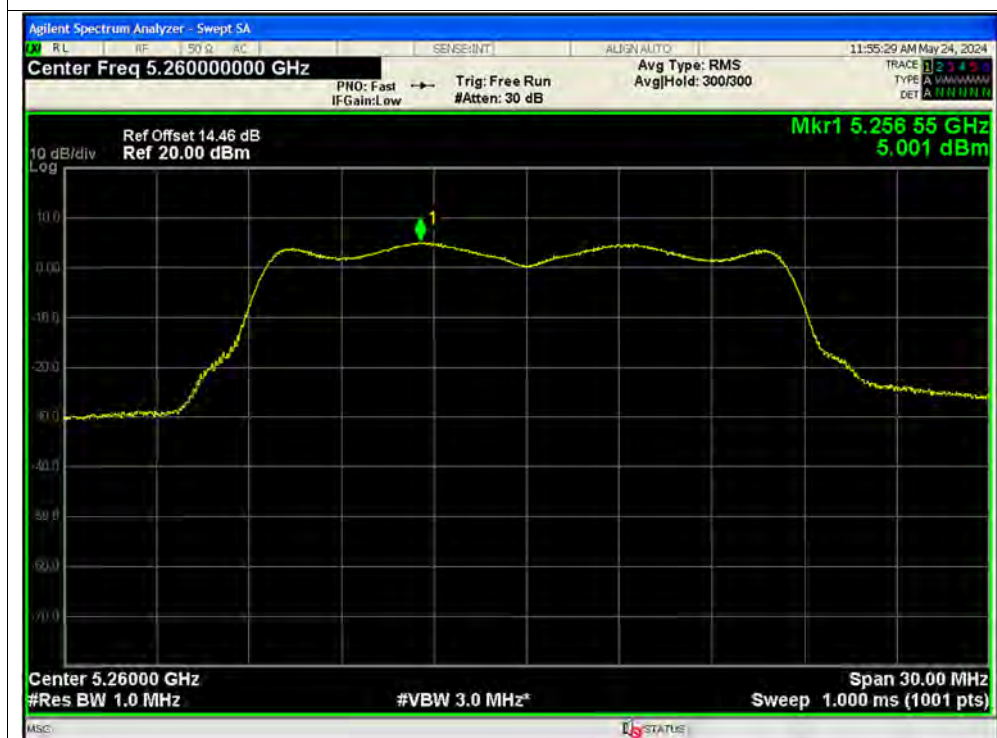
PSD NVNT a 5260MHz Ant1
