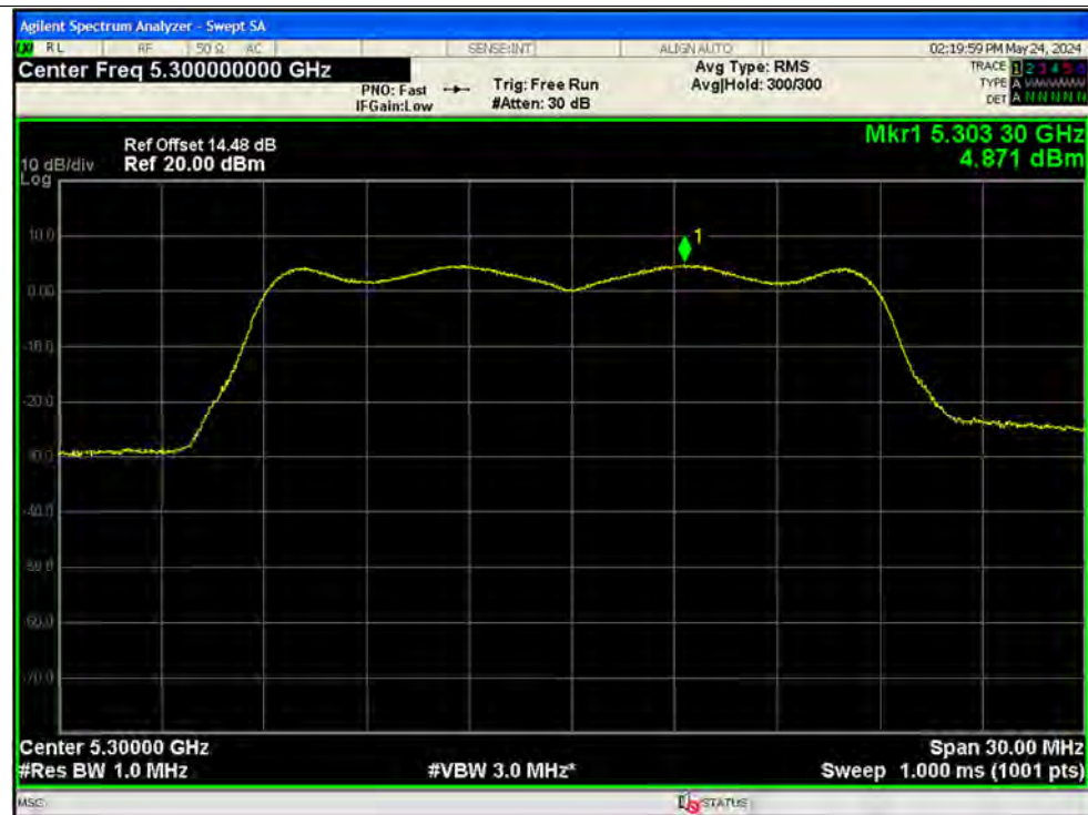
PSD NVNT n20 5300MHz Ant2
