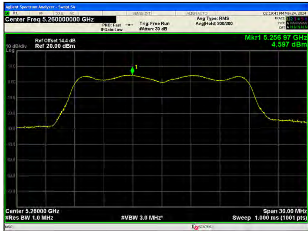
PSD NVNT n20 5300MHz Ant2
