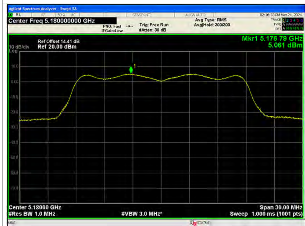
PSD NVNT n20 5180MHz Ant2
