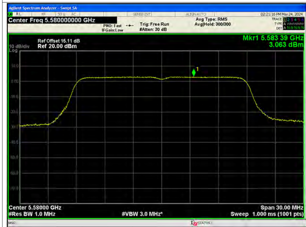
PSD NVNT n20 5600MHz Ant2
