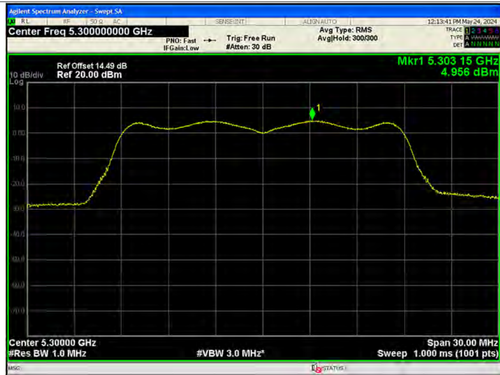
PSD NVNT n20 5320MHz Ant1
