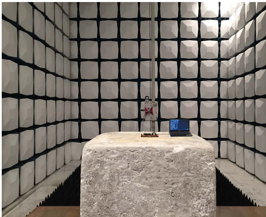
Description: Radiated Emission Test Setup for 1~18GHz
