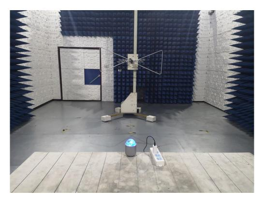
RADIATED EMISSION TEST SETUP ABOVE 1GHZ
