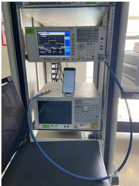
RF Conducted Test setup (BT/WIFI)
