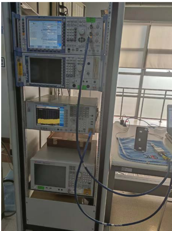
RF Conducted Test setup (GSM/WCDMA/LTE)
