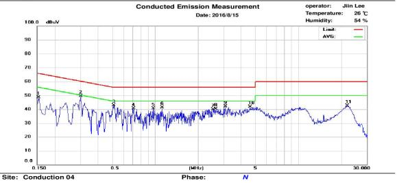
Limit: CISPR22 Class B Conduction(QP)
