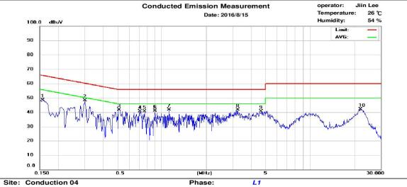
Limit: CISPR22 Class B Conduction(QP)
