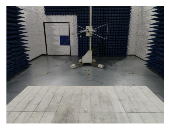
RADIATED EMISSION TEST SETUP ABOVE 1GHZ
