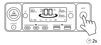
Press the ON/OFF button for 2 seconds to turn your power station on or off.
