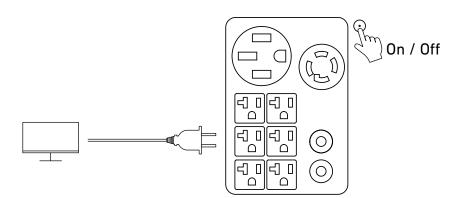
Double-click the AC outlet button, wait until the car icon appears on the screen, then connect your EV charge to the L14-30R or 14-50 AC output port.
