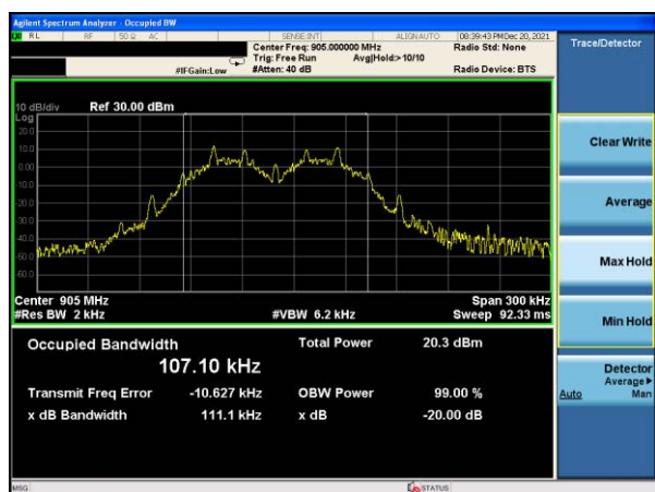
20dB Bandwidth plot on channel 01 (1Mbps)
