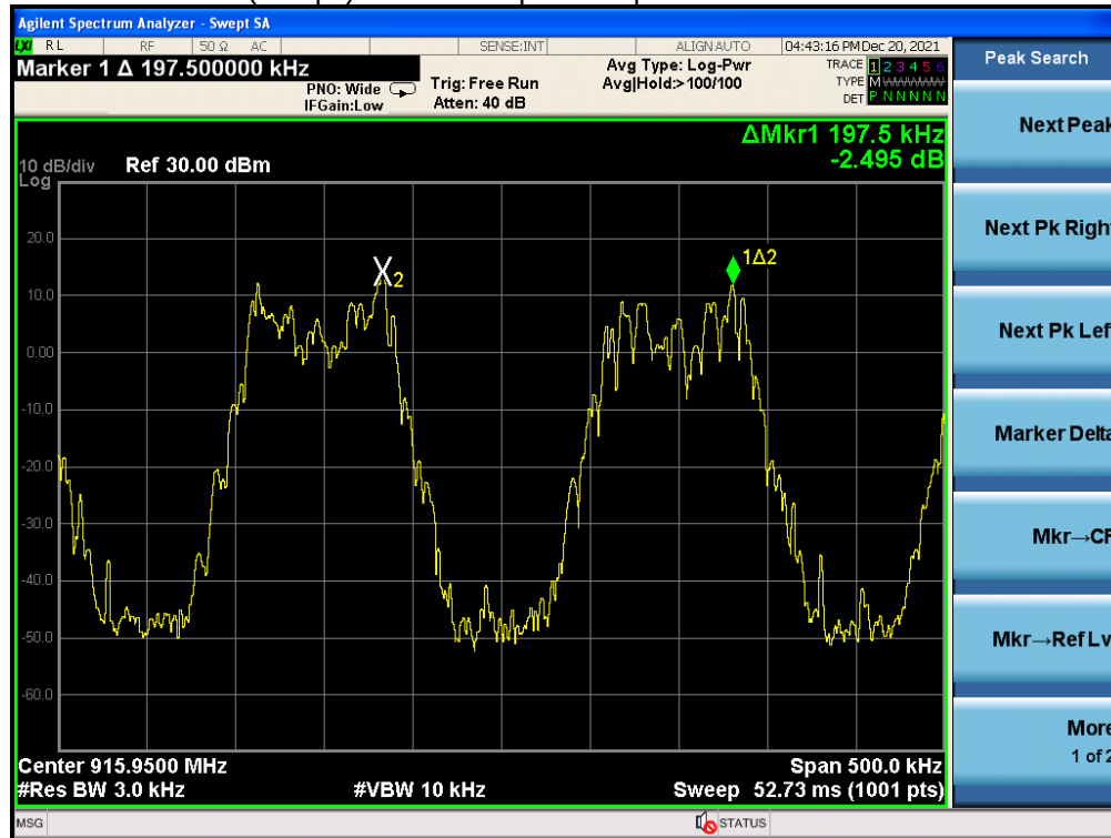
(1Mbps) Channel Separation plot on channel 102-103
