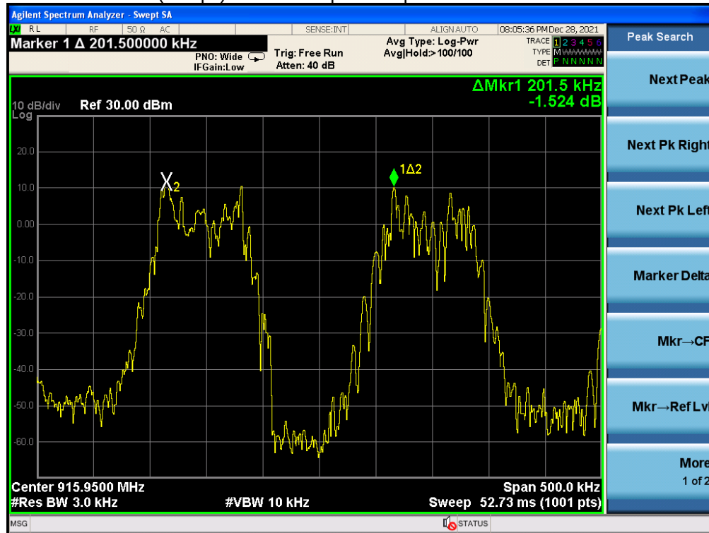
(1Mbps) Channel Separation plot on channel 102-103
