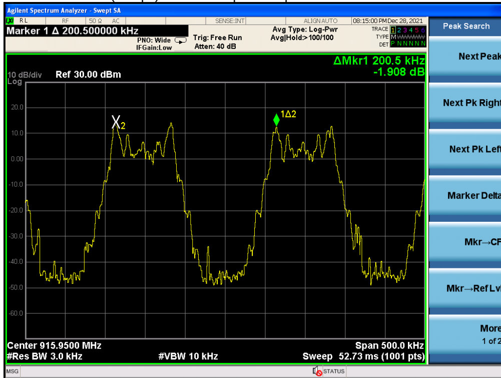
(1Mbps) Channel Separation plot on channel 102-103
