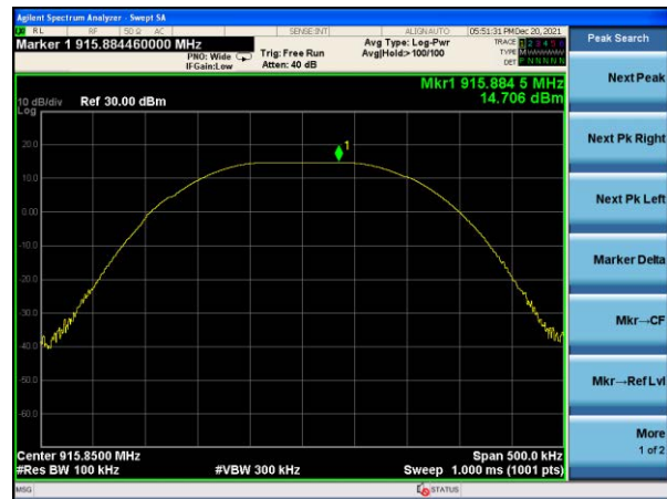
Peak output Power plot on channel 52 (1Mbps)
