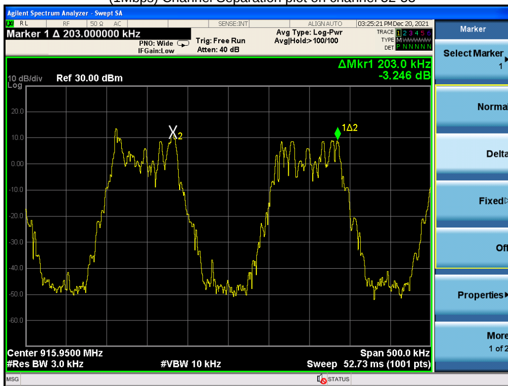
(1Mbps) Channel Separation plot on channel 102-103
