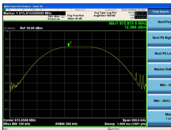
Peak output Power plot on channel 52 (1Mbps)
