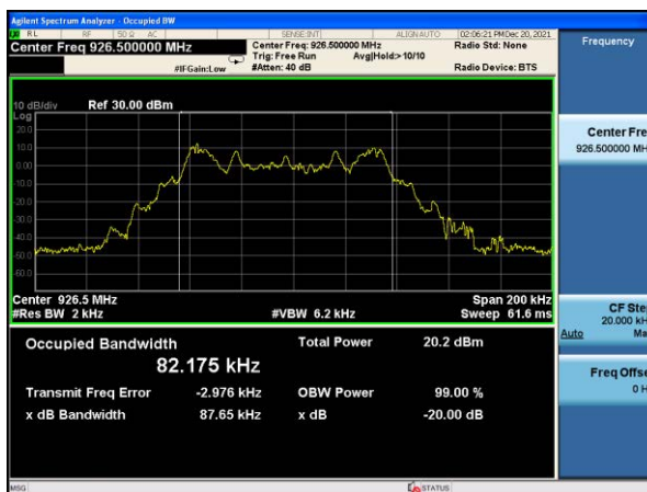
20dB Bandwidth plot on channel 103 (1Mbps)
