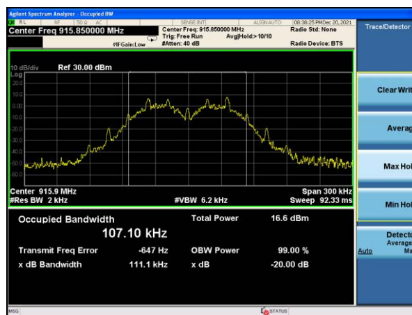
20dB Bandwidth plot on channel 52 (1Mbps)
