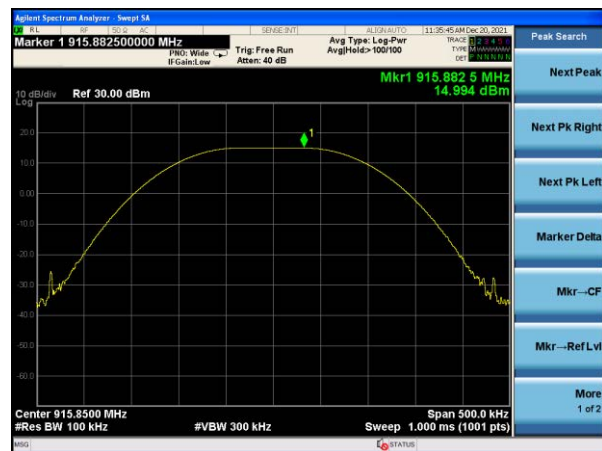
Peak output Power plot on channel 52 (1Mbps)
