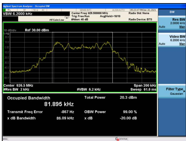
20dB Bandwidth plot on channel 103 (1Mbps)
