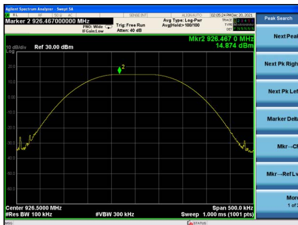
Peak output Power plot on channel 103 (1Mbps)
