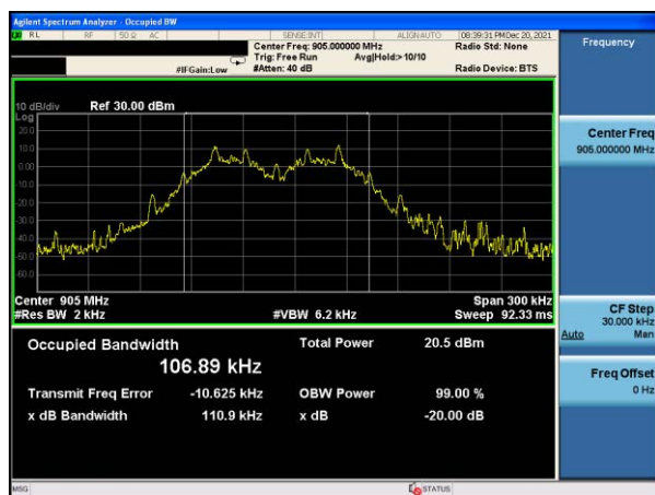
20dB Bandwidth plot on channel 103 (1Mbps)
