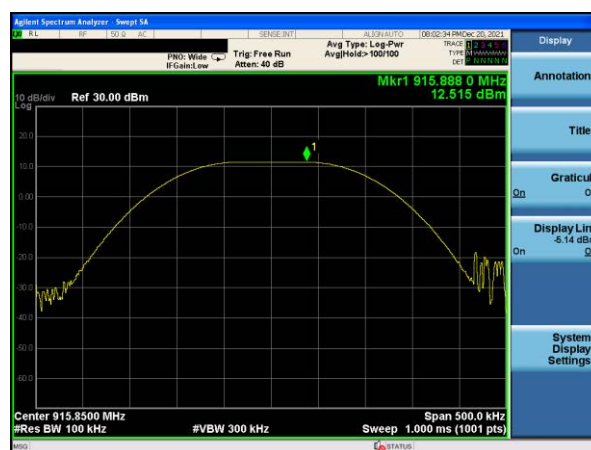
Peak output Power plot on channel 52 (1Mbps)
