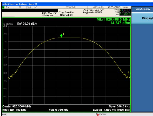
Peak output Power plot on channel 103 (1Mbps)
