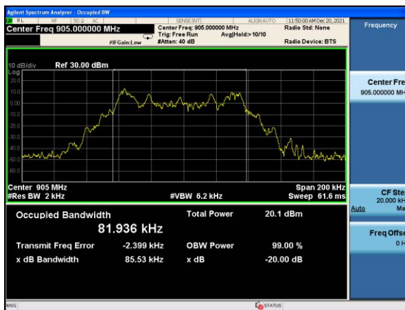
20dB Bandwidth plot on channel 103 (1Mbps)
