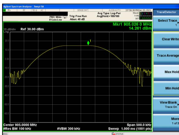
Peak output Power plot on channel 01 (1Mbps)
