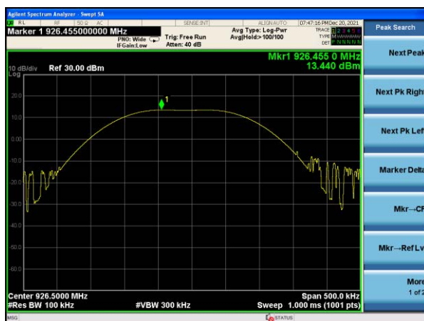
Peak output Power plot on channel 103 (1Mbps)
