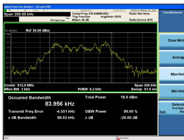
20dB Bandwidth plot on channel 52 (1Mbps)
