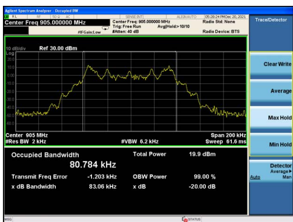
20dB Bandwidth plot on channel 01 (1Mbps)
