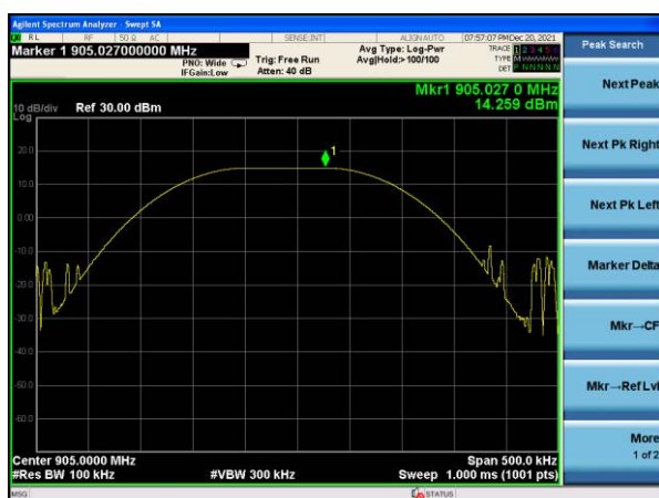
Peak output Power plot on channel 01 (1Mbps)
