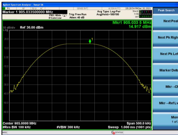
Peak output Power plot on channel 01 (1Mbps)
