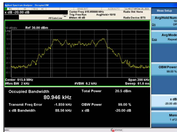
20dB Bandwidth plot on channel 52 (1Mbps)
