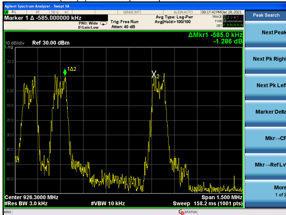
(1Mbps) Channel Separation plot on channel 102-103
