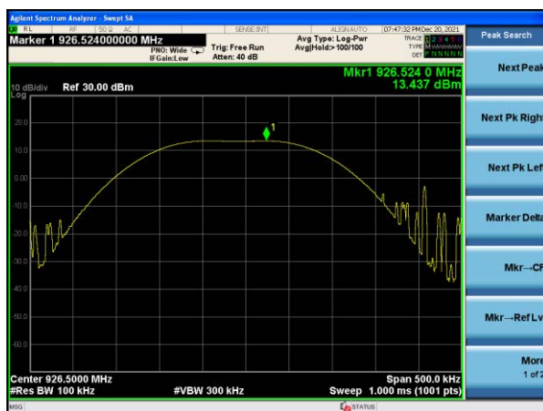
Peak output Power plot on channel 103 (1Mbps)
