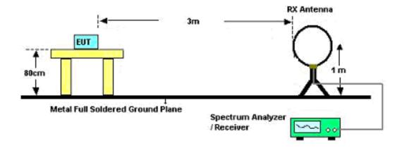
For Radiated Emissions: 30MHz~1GHz
