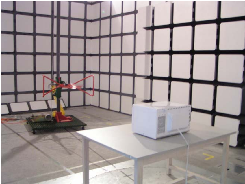
Radiated Emission (30MHz to 1000MHz) - Rear View
