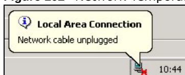
Figure 102 Network Temporarily Disconnected
