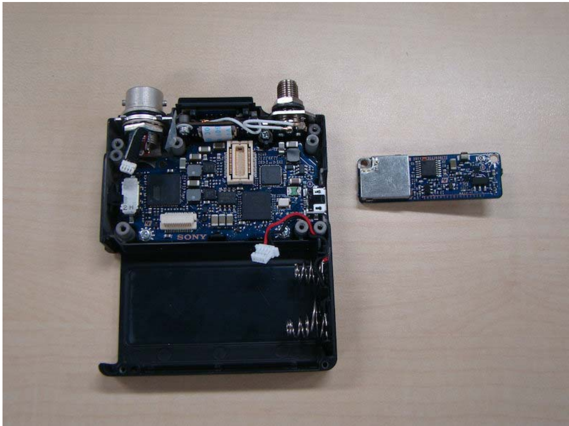
Fig.5: Removed the board TX-147
