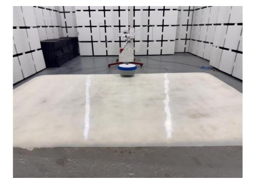
Set-up for Radiated Spurious Emission, Below 1GHz
