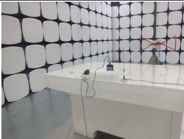
Radiated Spurious Emissions Test Setup Below 1GHz
