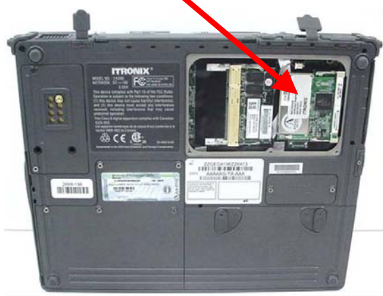
Photograph A-3 - WLAN Mini-PCI Card Location
