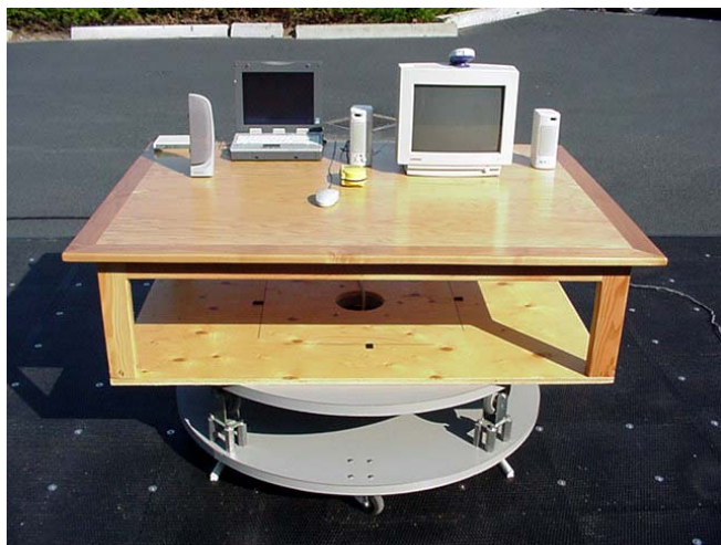
Photograph F-2 - Front of Radiated Emission Configuration
