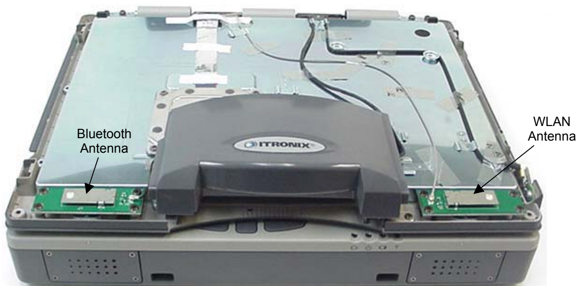
Photograph A-7 - Surface Mount Antenna Placement
