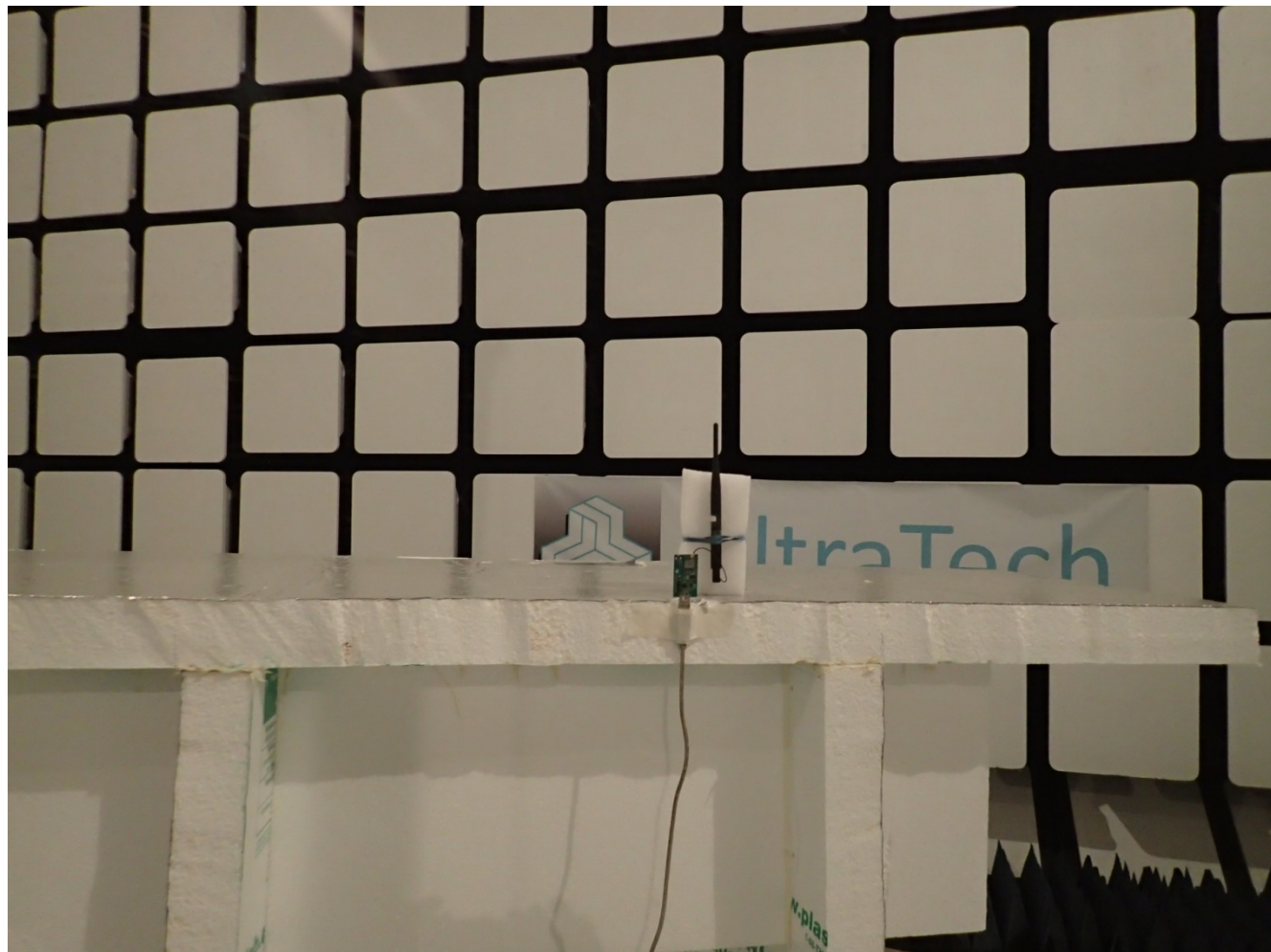
Radiated Emissions @ 3 m, Orthogonal Position 3
