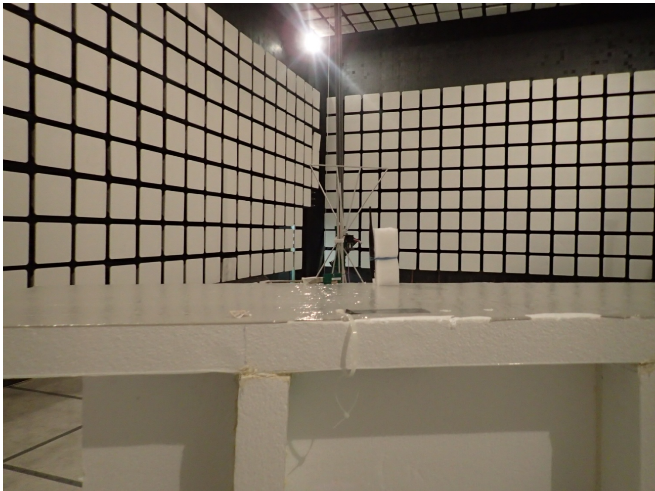
Radiated Emissions @ 3 m, Orthogonal Position 2
