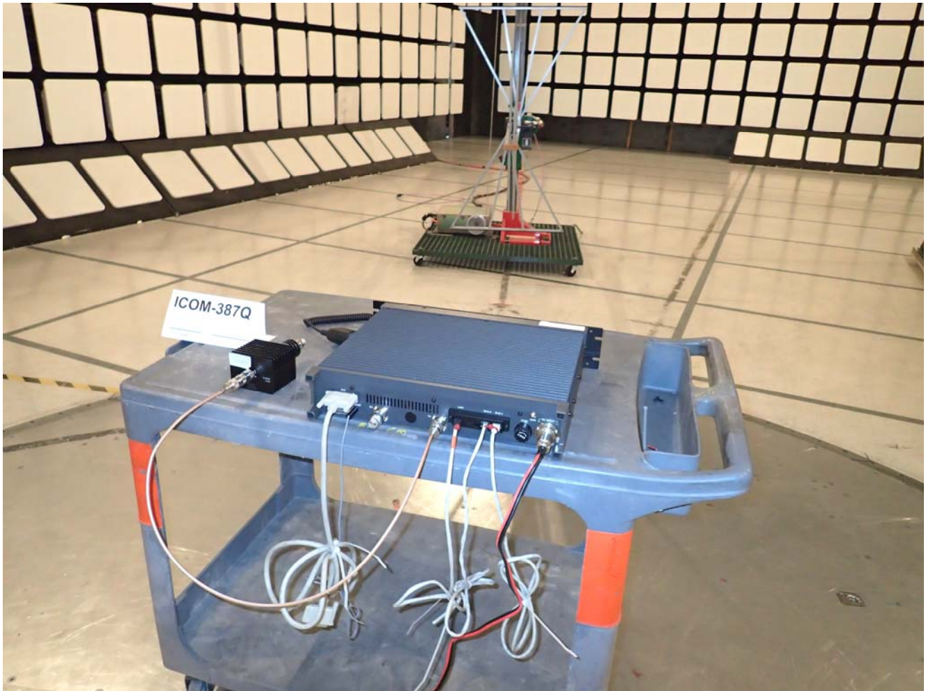
Plot #3: Tx Radiated Emission Test Setup
