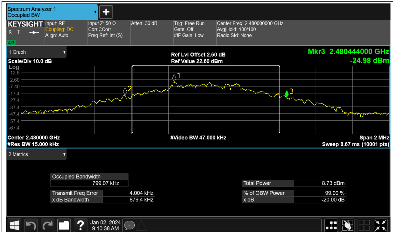
-20dB Bandwidth NVNT 2-DH1 2402MHz Ant1
