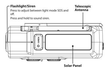
**Note:** The solar panels charge at a very slow rate. Therefore, it is best used as a supplemental charging method in addition to the charging cable
