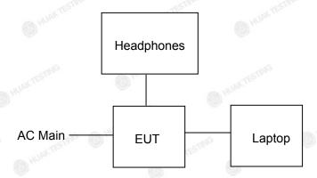
Operation of EUT during Radiation Above 1GHz testing:
