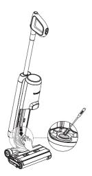
Clean the dirt sensor with a damp cloth or the cleaning tool.
