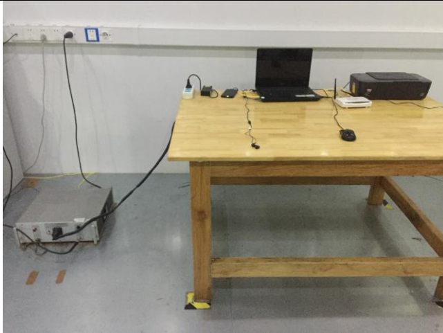
Conducted Emissions Test Setup – Front View
