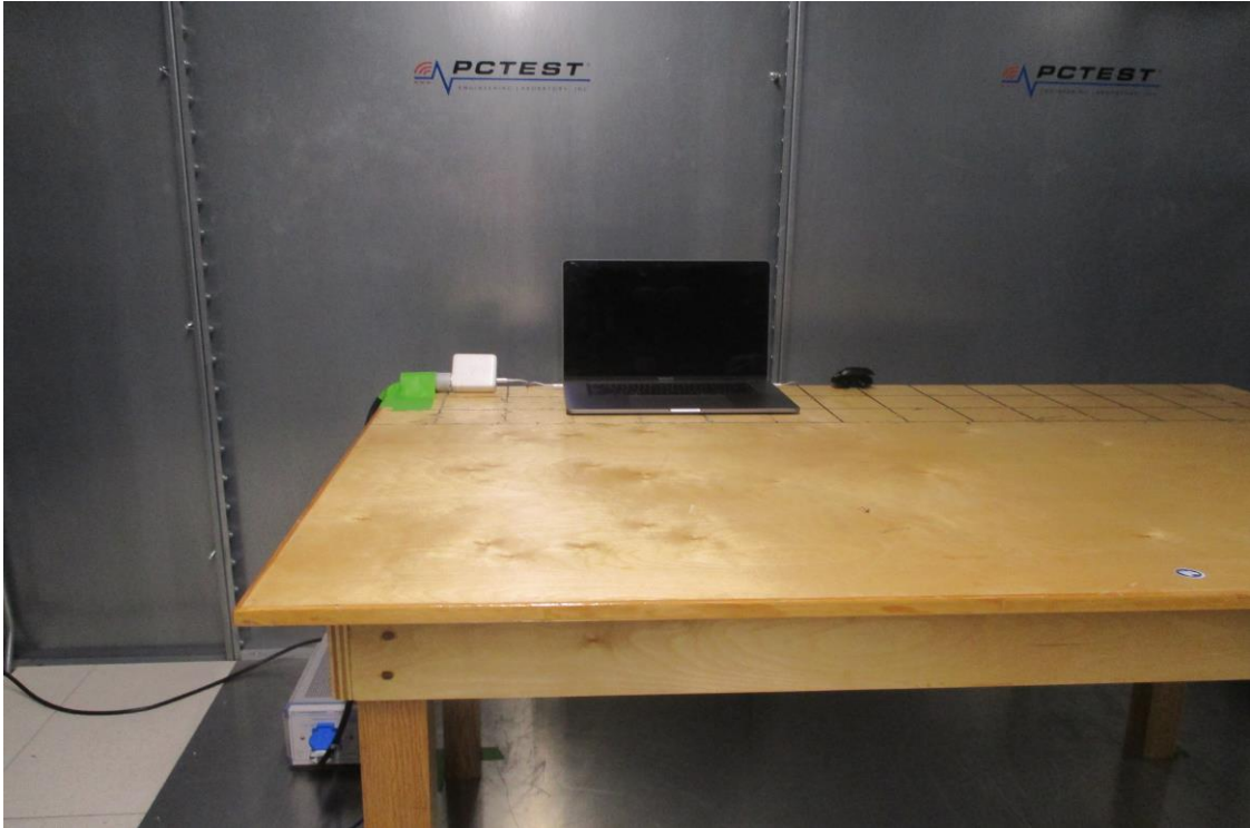
Figure 15: AC Line Test Setup (Front View)
