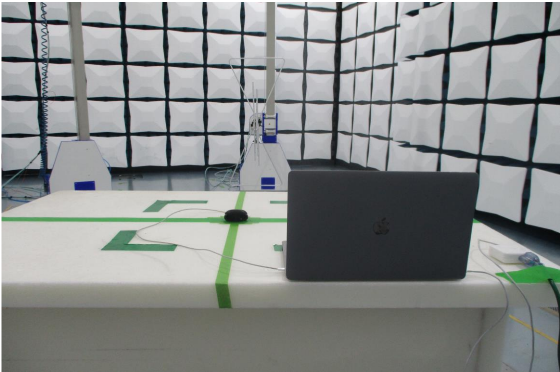
Figure 12: 30MHz-1GHz Test Setup (Rear View)
