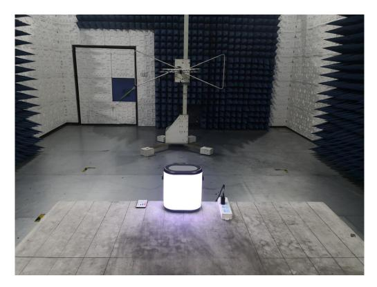
RADIATED EMISSION TEST SETUP ABOVE 1GHZ
