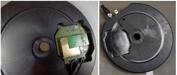
The coil wire is covered with potting during final manufacturing steps.
