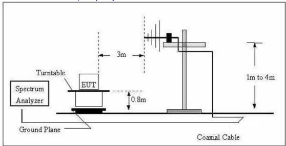
(C) Radiated Emission Test-Up Frequency Above 1GHz
