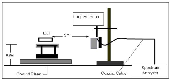
2. Radiated Emission Test-Up Frequency Below1GHz
