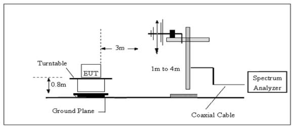
3. Radiated Emission Test-Up Frequency Above 1GHz
