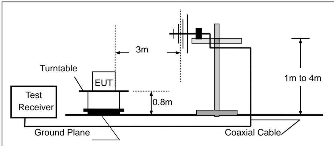
(C) For radiated emissions above 1000MHz
