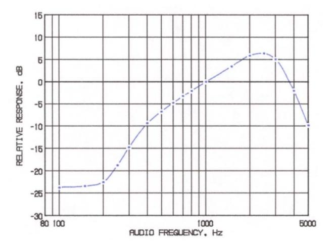
MODULATION FREQUENCY RESPONSE FCC ID: BBOPR950DXD
