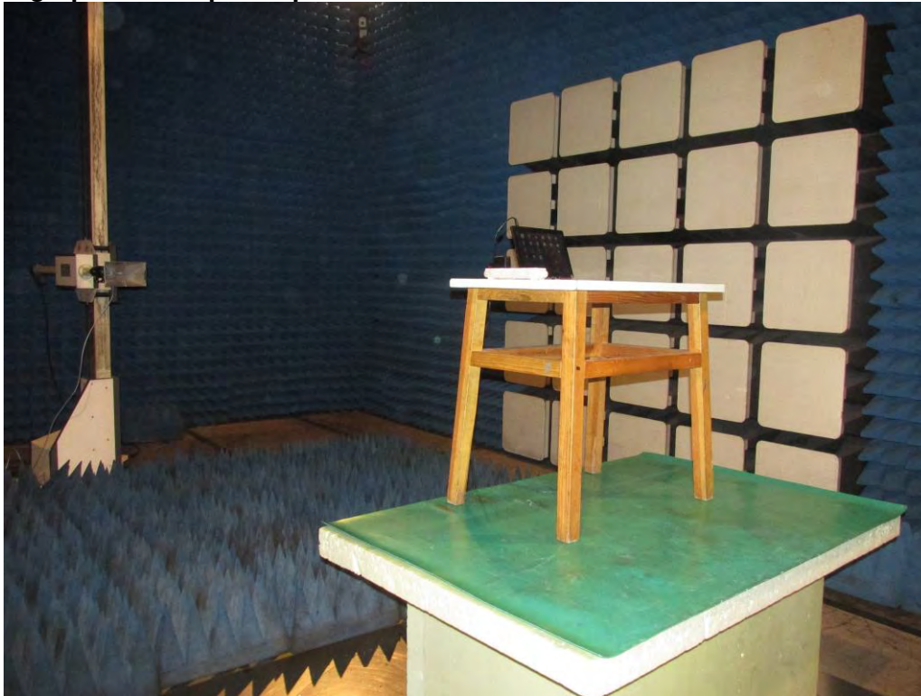
Photograph 4: Set-up for Spurious Emissions for 18 - 26.5GHz
