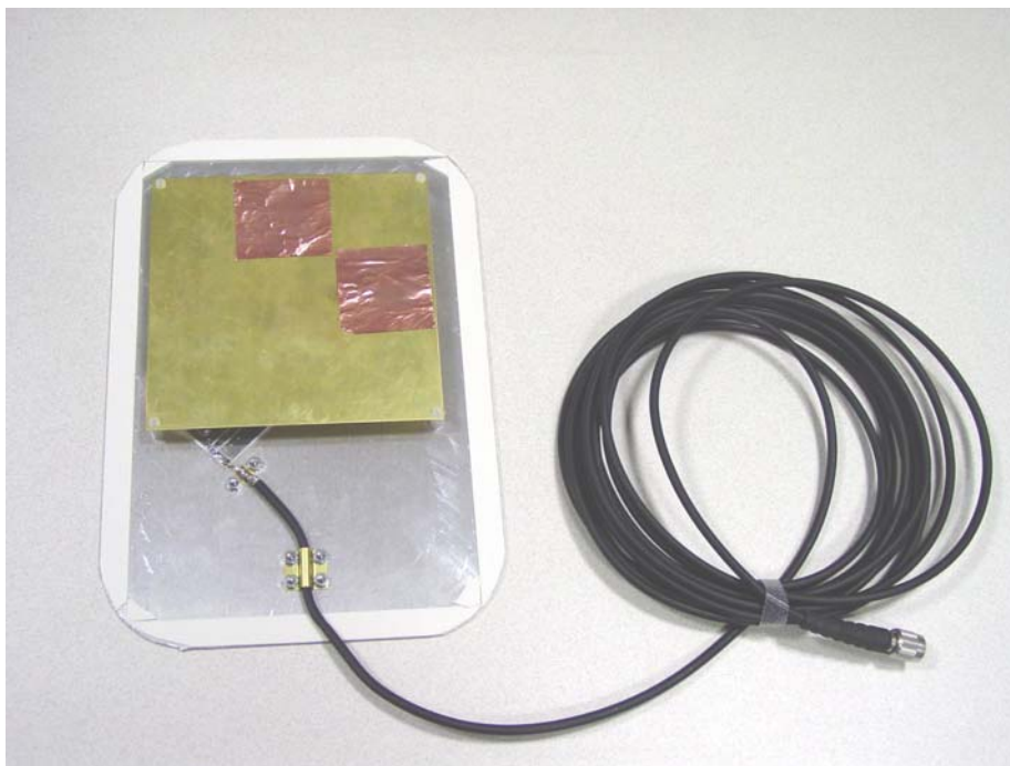
Circular Antenna Internal View
