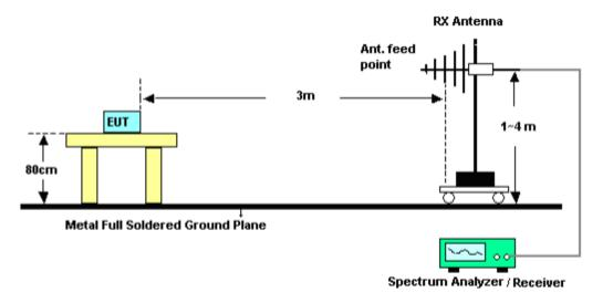
(C) Radiated Emission Test-Up Frequency Above 1GHz
