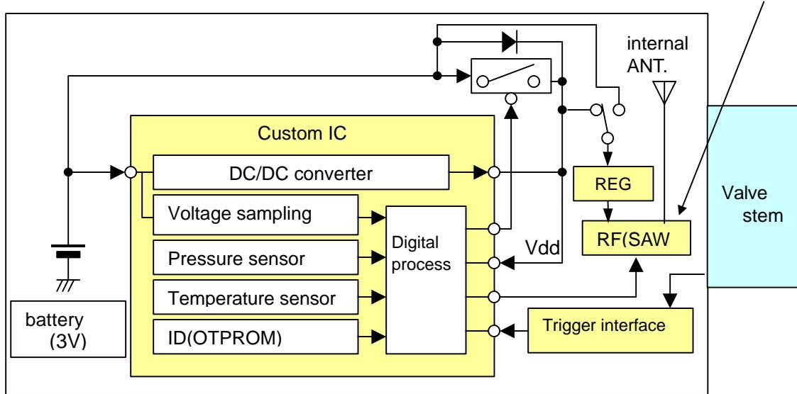
Fig 6, Block diagram of transmitter
