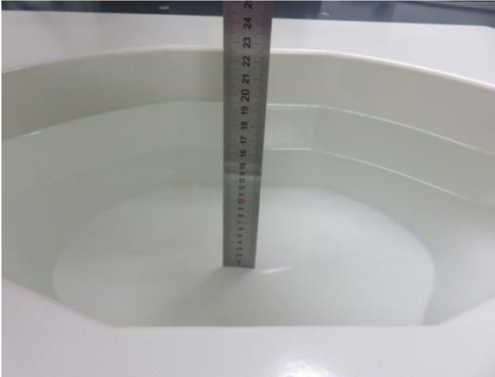
Photograph of the depth in the Body Phantom (5800MHz, 16.1cm depth)
