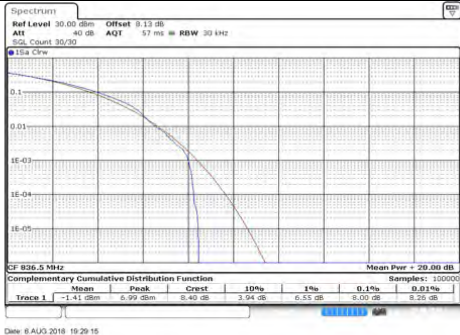
Peak-Average Ratio Plot(5MHz BW,QPSK,Band 5-mid Channel)
