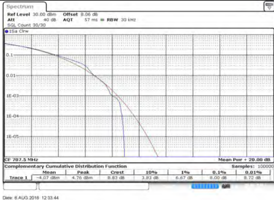
Peak-Average Ratio Plot(10MHz BW,QPSK,Band 12-mid Channel)
