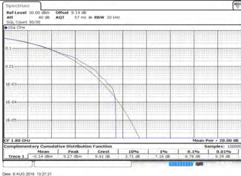
Peak-Average Ratio Plot(3MHz BW,QPSK,Band 2-mid Channel)
