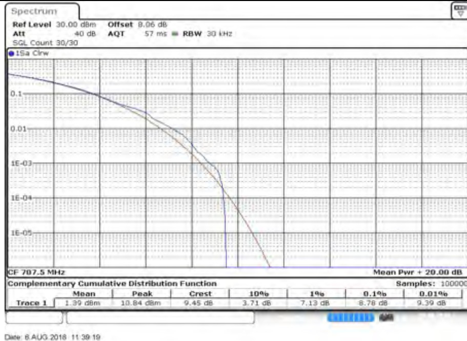
Peak-Average Ratio Plot(3MHz BW,QPSK,Band 12-mid Channel)
