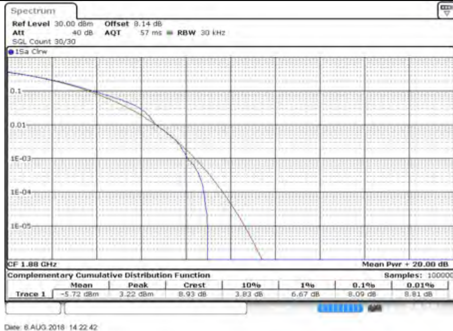
Peak-Average Ratio Plot(10MHz BW,QPSK,Band 2-mid Channel)
