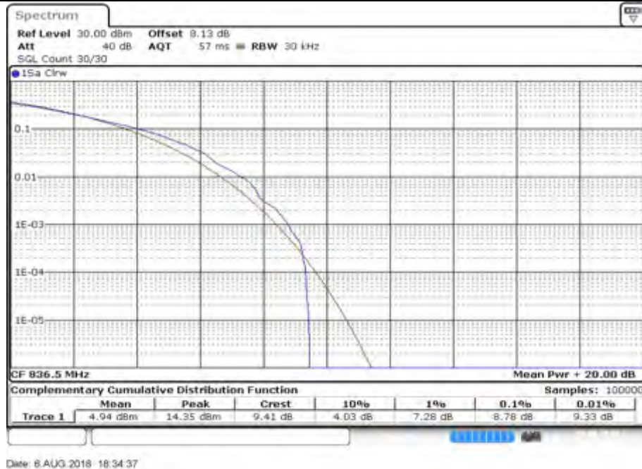
Peak-Average Ratio Plot(1.4MHz BW,QPSK,Band 5-mid Channel)
