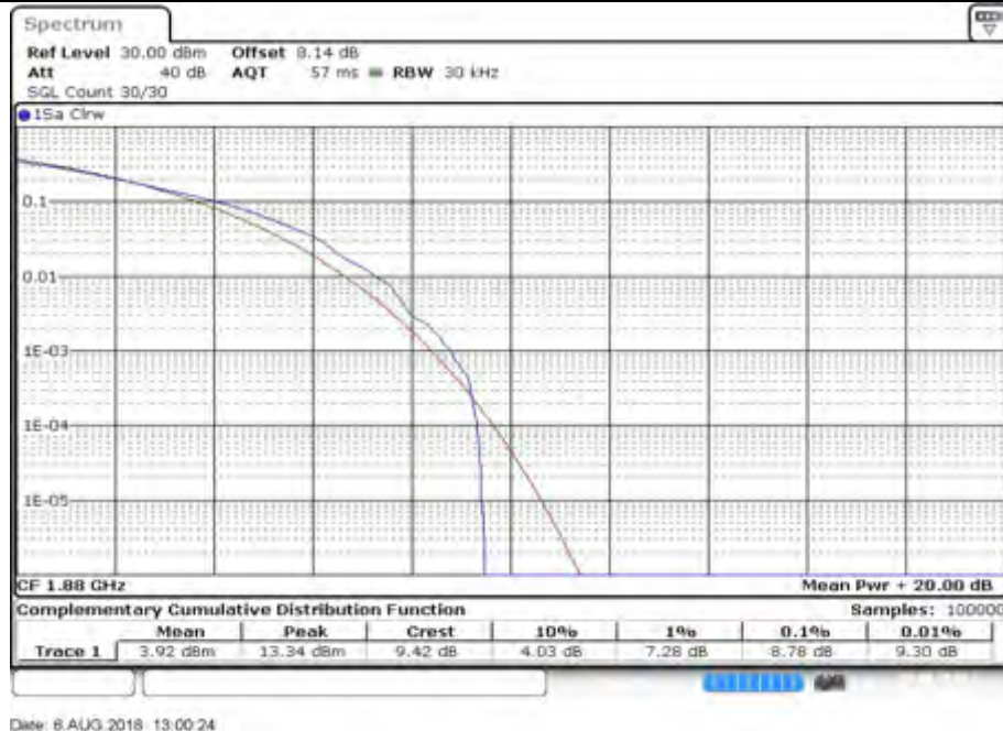
Peak-Average Ratio Plot(1.4MHz BW,QPSK,Band 2-mid Channel)
