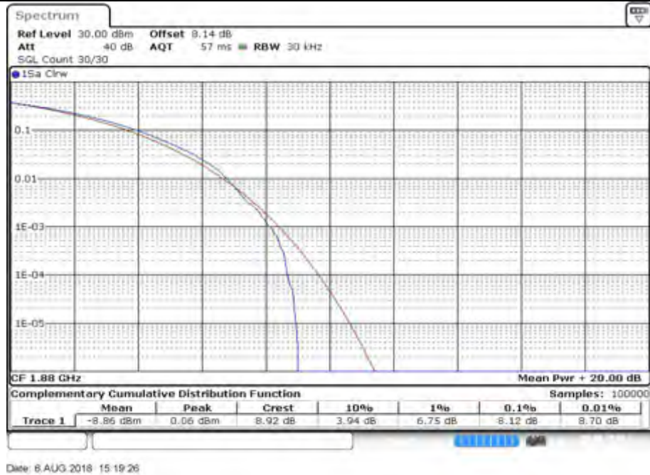
Peak-Average Ratio Plot(20MHz BW,QPSK,Band 2-mid Channel)
