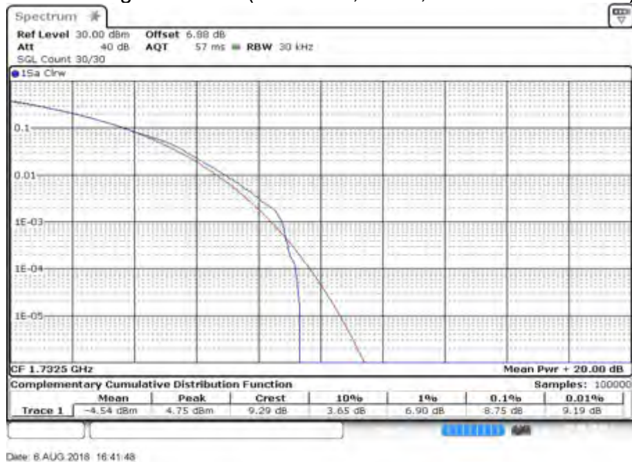
Peak-Average Ratio Plot(5MHz BW,16QAM,Band 4-mid Channel)
