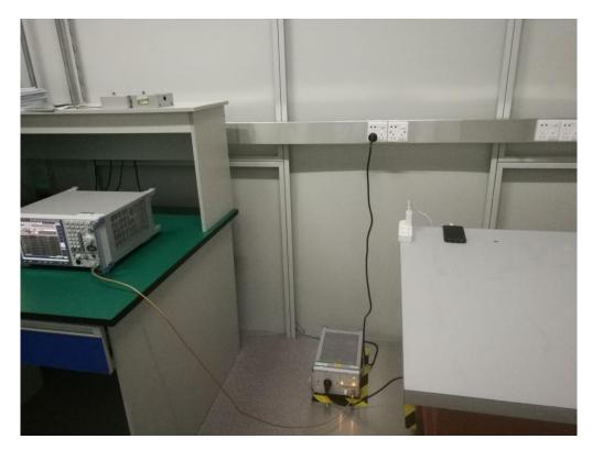
RADIATED EMISSION TEST SETUP
