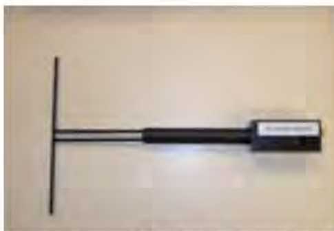
Figure 1 – Satimo COMOSAR Validation Dipole
