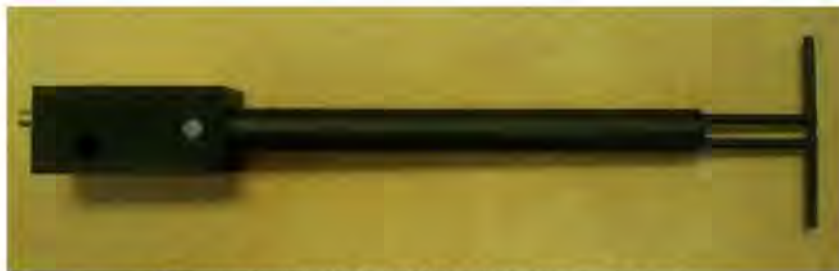
Figure 1 – MVG COMOSAR Validation Dipole
