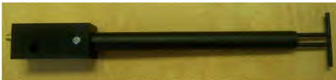
Figure 1 – MVG COMOSAR Validation Dipole
