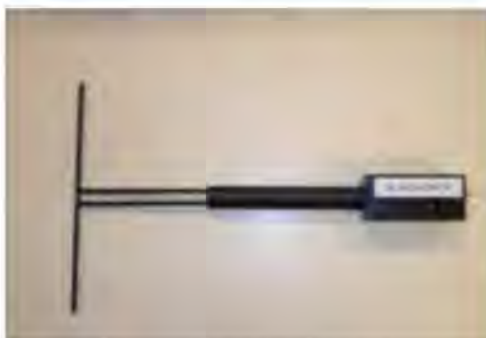
Figure 1 – Satimo COMOSAR Validation Dipole
