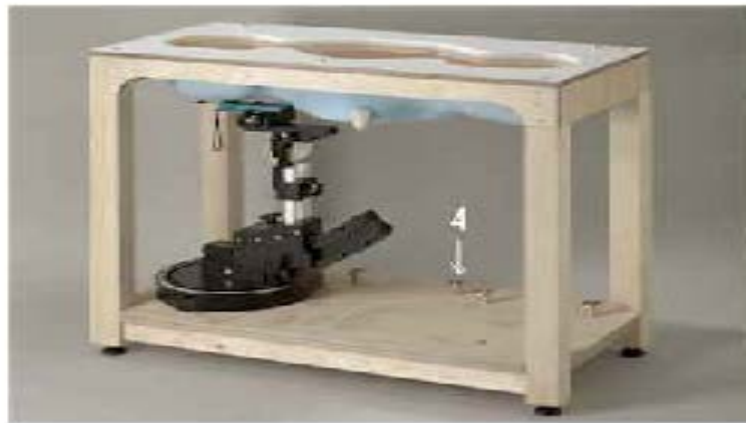
Figure 5.0-1 SAM Twin Phantom
