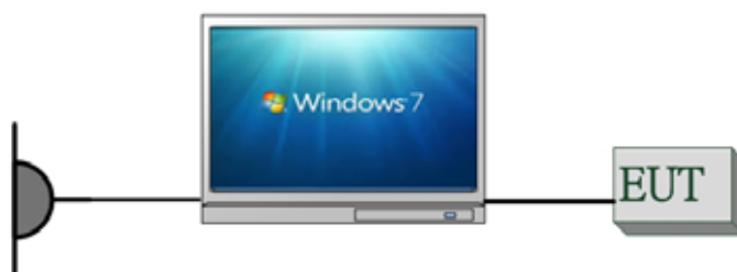
Fig. 2-2 Radiated Emission Configuration (NFC)
