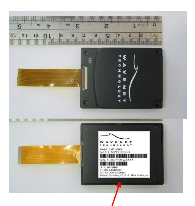
Label is placed in recess on rear of modem
